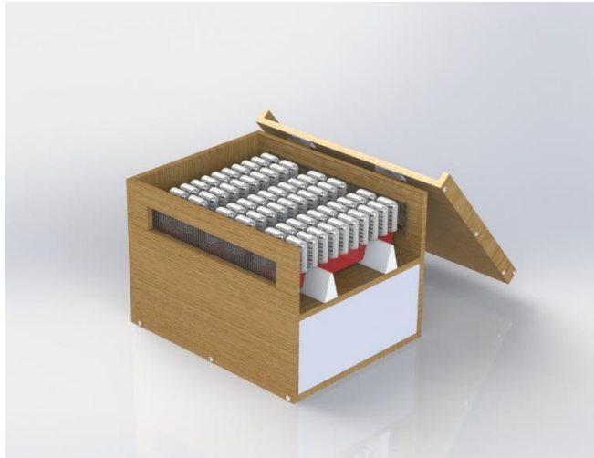
Figure 2: PPC Design with Lid Open with Right Panel Removed (437mm x 284mm x 246mm)
