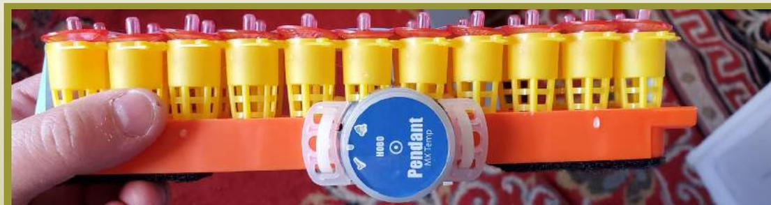
Figure 15. An Onset HOBOT Pendant® MX2201 temperature data logger attached to a JZs BZs shipping bar.
